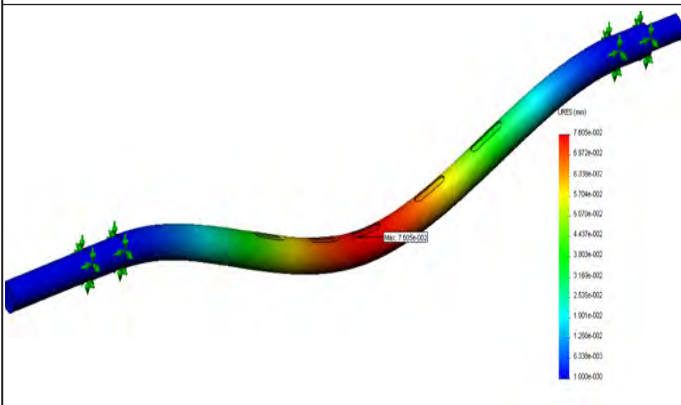
FEM analysis (shaft sample)
