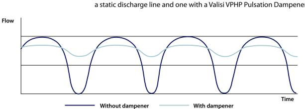
The following graph shows the difference in efficiency between a system with a static discharge line and one with a Valisi VPHP Pulsation Dampener:
