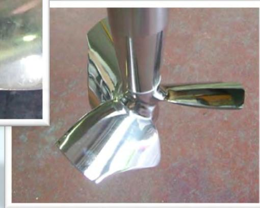
*For impeller  $\varnothing > 600$  mm blades to be welded within vessel*
